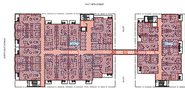
3RD FLOOR BUILDING A TOTAL AREA FACTORED INTO GROSS F.A.R. CALCULATION: 12010 SF + 113 SF = 12123 SF BUILDING B TOTAL AREA FACTORED INTO GROSS F.A.R. CALCULATION: 5338 SF + 113 SF = 5451 SF BUILDING A TOTAL AREA FACTORED INTO NET F.A.R. CALCULATION: 11904 SF BUILDING B TOTAL AREA FACTORED INTO NET F.A.R. CALCULATION: 4433 SF
